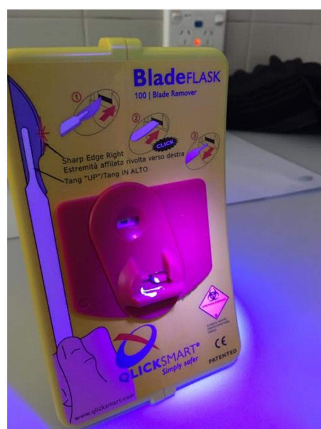
Fig 2. Contaminated interior and aperture after removal
