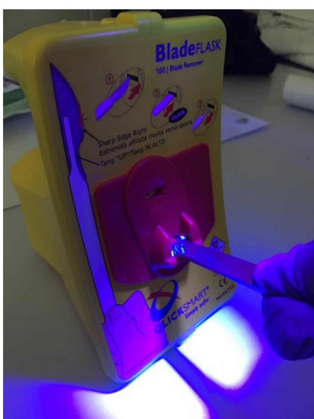
Fig 1. Contaminated blade and handle inserted into SBR
